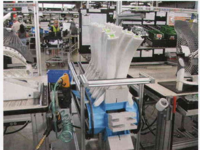
'FLIP-OVER' CONCEPT. The packaging's flip-over concept allows filler to automatically index to the next available spine every time one is removed by the operator.
